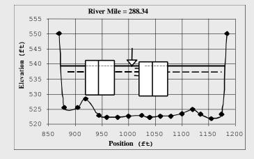
The pool is very narrow (105 m) with vertical concrete or sheet pile embankments and fencing.
