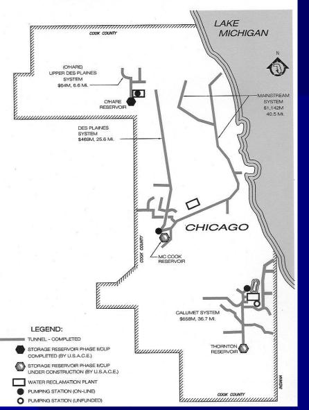
More than 150 km of 12 meter diameter underground tunnels were built (drilled) to store and subsequently treat combined and sanitary sewer overflows
